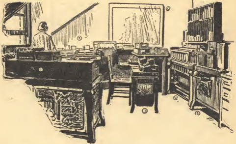
Fig. 1. The astronomical calculating machines used by the Columbia University Department of Astronomy. This apparatus is assembled from various International Business Machine calculating and bookkeeping units, slightly modified for the work of astronomers. The numbered units are (1.) the multiplier, (2.) tabulator, (3.) summary punch, (4.) card sorter, (5.) high speed reproducer, and (6.) blackboard for notes and instructions for workers on the next shift. To this machine, the cards are memory, the sorter the ability to select a given fact from the mass of knowledge in memory, et cetera.
