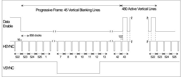
Figure 5. Timing parameters for 720x480p @ 59.94/60 Hz.
