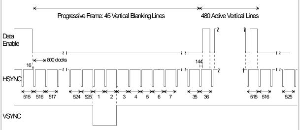
Figure 2. Timing parameters for 640x480p @ 59.94/60 Hz.
