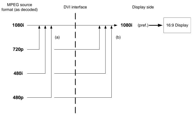
Figure 26. Example of options for format conversion
