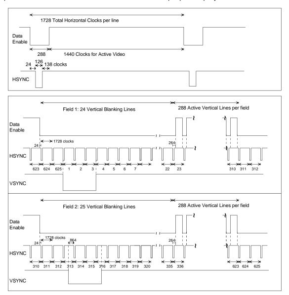
Figure 10. Timing Parameters for 720(1440)x576i @ 50 Hz
