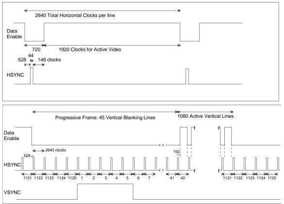
Figure 23. Timing Parameters for 1920X1080p @ 29.97/30 Hz.
