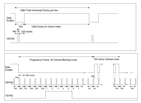
Figure 7. Timing parameters for 1280x720p @ 50 Hz.
