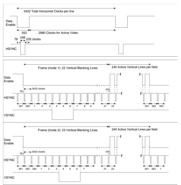
Figure 13. Timing Parameters for (2880)X240p @ 59.94/60 Hz.
