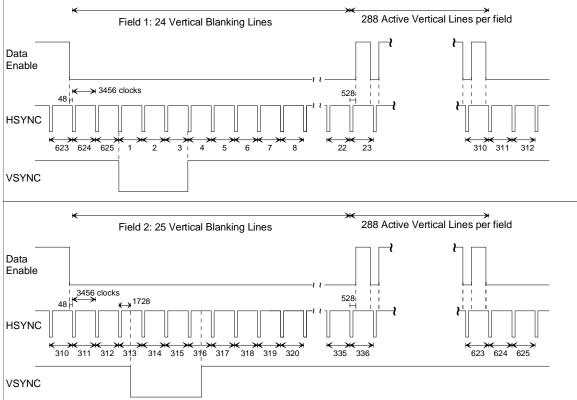
Figure 17. Timing Parameters for (2880)X576i @ 50 Hz
