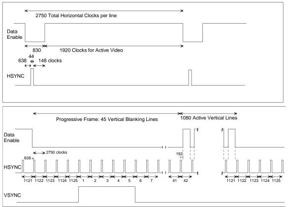
Figure 21. Timing Parameters for 1920X1080p @ 23.97/24 Hz.
