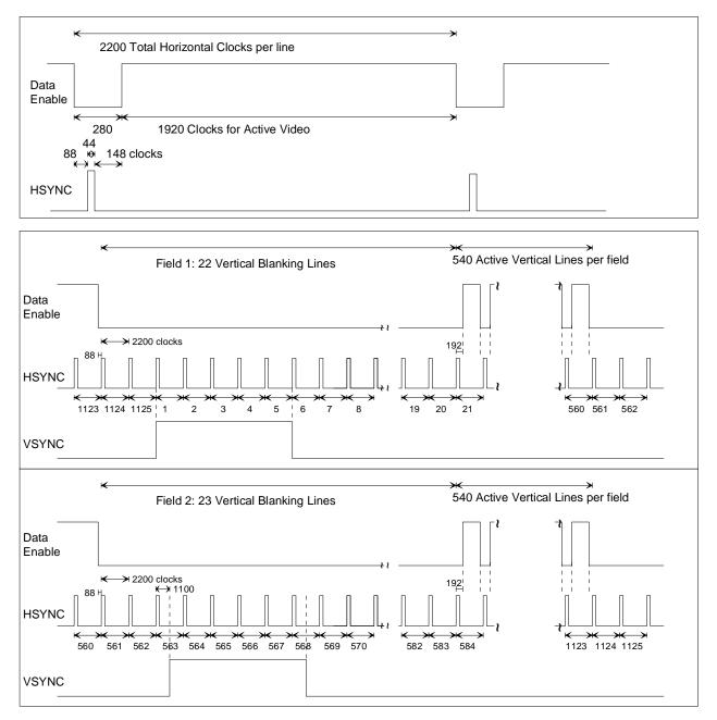
Figure 4. Timing parameters for 1920x1080i @ 59.94/60 Hz.
