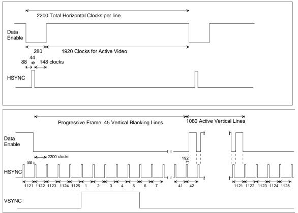
Figure 15. Timing Parameters for 1920X1080p @ 59.94/60 Hz.
