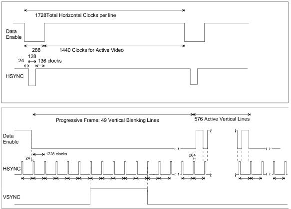
Figure 19. Timing Parameters for 1440X576p @ 50 Hz.
