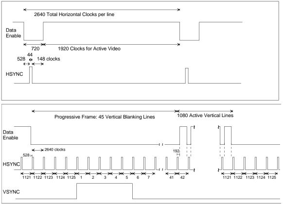
Figure 20. Timing Parameters for 1920X1080p @ 50 Hz.
