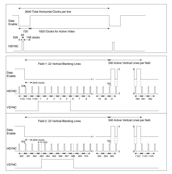
Figure 8. Timing parameters for 1920x1080i @ 50 Hz.
