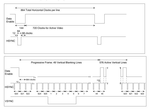
Figure 9. Timing parameters for 720x576p @ 50 Hz.
