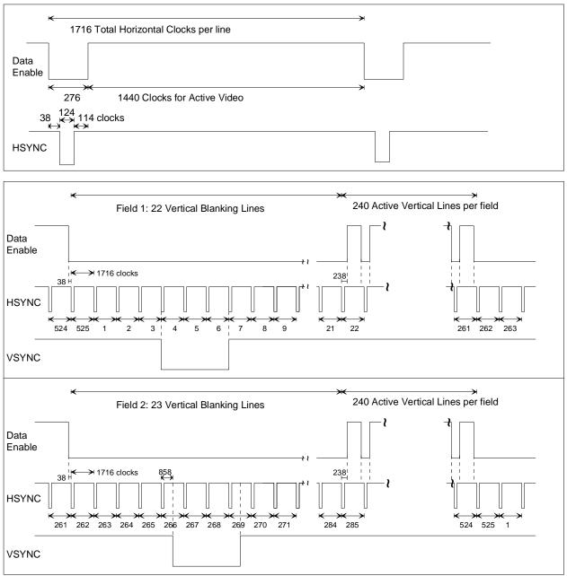
Figure 6. Timing Parameters for 720(1440)X480i @ 59.94/60 Hz.
