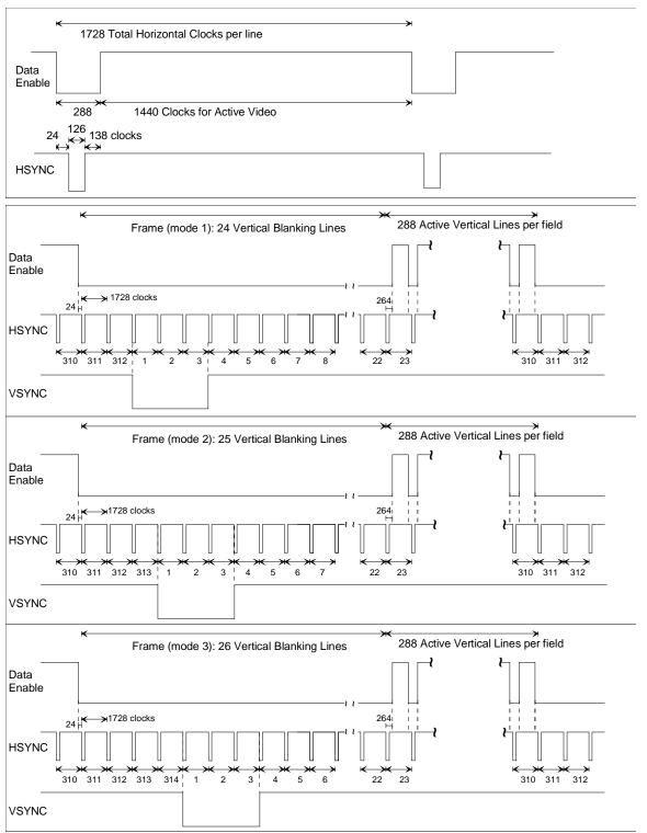
Figure 16. Timing Parameters for 720(1440)X288p @ 50 Hz.
