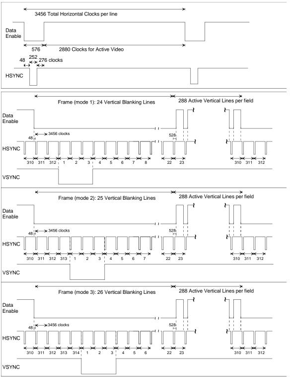
Figure 18. Timing Parameters for (2880)X288p @ 50 Hz.
