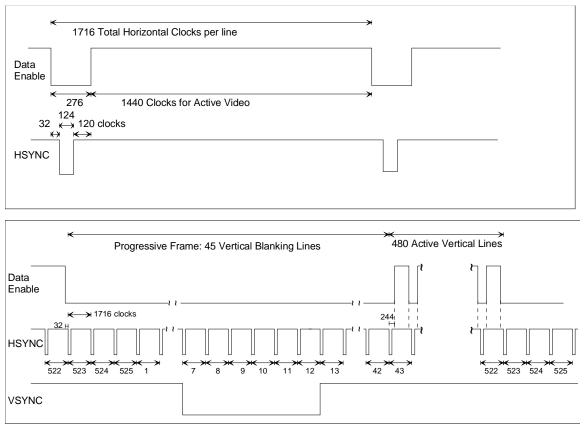
Figure 14. Timing Parameters for 1440X480p @ 59.94/60 Hz.
