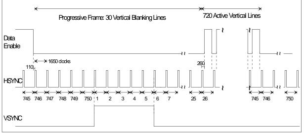
Figure 3. Timing parameters for 1280x720p @ 59.94/60 Hz.
