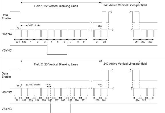
Figure 12. Timing Parameters for (2880)X480i @ 59.94/60 Hz.
